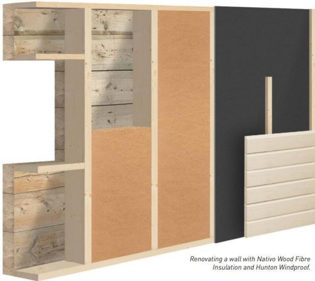
*Renovating a wall with Nativo Wood Fibre Insulation and Hunton Windproof.*
